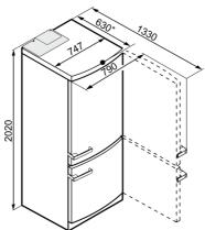
\*To ensure that energy consumption as stated is achieved, machines should be used together with the enclosed spacer brackets. This increases the total depth of the unit by approx. 3.5 cm. , Machines are still fully functional when operated without these brackets but have a slightly higher energy consumption.,
